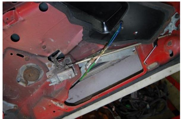
12. Connect the door lock actuator wires to the door lock harness (wire color may be different than photo). Connect the numerals together found on harness and door lock actuators 1-1 2-2.
