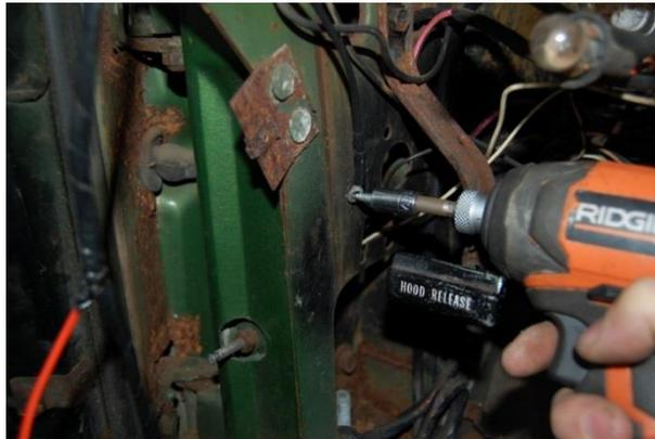
21. The black wire should be grounded to the metal framework under the kick panel.
