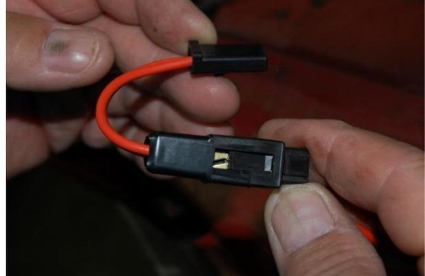
18. We provide an additional 56 series male connector in the female connector to protect the terminal. If you already have an accessory that requires battery power plugged into the fuse panel at this position, the male connector is removed from the female connector for installation onto your existing accessory, per supplied photos.
