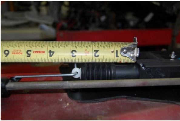
15. A good indicator that the lock linkages are working correctly- the door lock actuator in the unlocked position is at 2.750".
