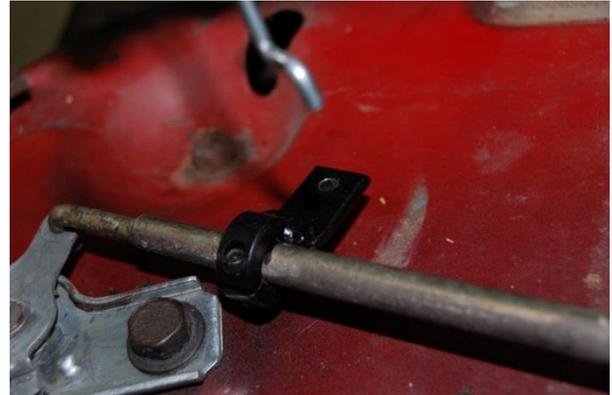
10. Before installing the access plate, remove the O.E. door lock horizontal external linkage clip at the bell crank (closest to the rear of the door), slip the supplied linkage adapter with the hex screw pointing upward onto the linkage rod until it stops, and tighten slightly (leave somewhat loose for adjustment purposes).
