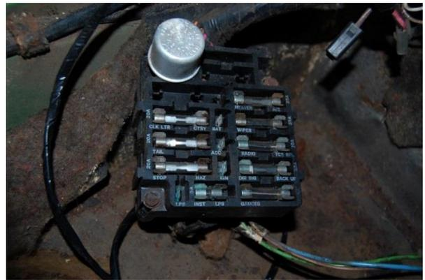
16. All 1968-1977 O.E. Corvette fuse panels have an auxiliary battery terminal for add-on battery powered accessories. The auxiliary battery terminal is protected via the courtesy fuse; no additional fuse is required. **If you decide to connect directly to the battery or other non-fused battery source a 20 amp fuse device must be connected to the orange battery power door lock system wire.**
