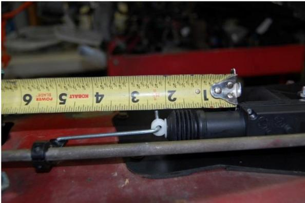
13. Adjustment of the O.E. lock linkage rod is next and **important for proper operation and door lock actuator life**. The door lock actuator rod should not bottom out in the door lock actuator housing when the lock is adjusted properly. There should be 2.125" from the rod end eye to the square portion of the door lock actuator housing when in the door locked position.
