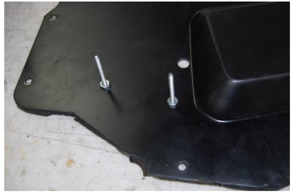
8. Install the provided 6-32x1.5" screws into the access panel, secure with the hex nuts and tighten (nuts are provided to keep the screws in place for simple actuator installation).
