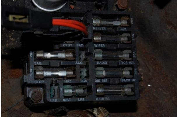
17. The power door lock harness **orange batt power wire lead** should be connected to the fuse panel auxiliary battery terminal.
