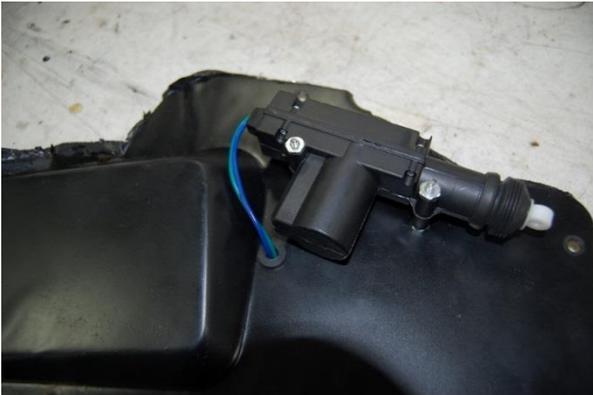
9. Place the actuator onto the screws installed into the access plate. Install the flange nuts and tighten to hold the actuator in place. Install the rubber grommet onto the lock actuator wire leads, place the door lock actuator wires through the access plate and install the rubber grommet.
