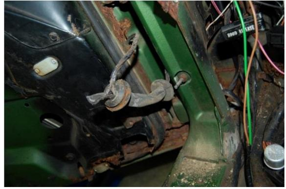
4. Remove the power window conduit from the door and door pillar. It is much easier to feed the door lock wiring through the rubber conduit once it is pulled away from the door and pillar. Feed the wiring through the upper door pillar hole, then the rubber conduit, and finally feed the wiring into the door.
