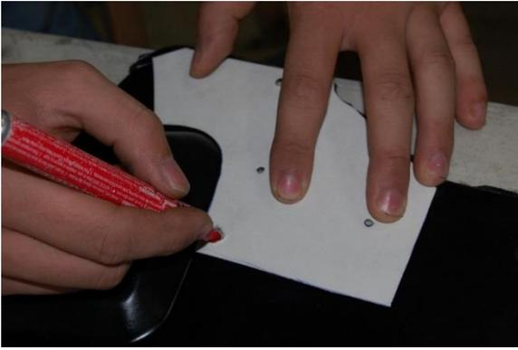
7. The template provided is to be placed onto the window regulator access plate to mark the drill location of the door lock actuator screws and wiring grommet. Center punch at your marks, drill two 9/64 holes in the plate for the door lock actuator and one 23/64 hole for the grommet. The same template is used for both doors, simply turned over for the appropriate
