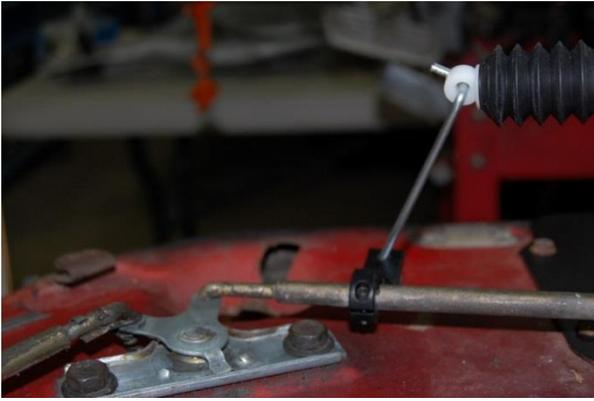
11. If the door lock actuator linkage has come out of the door lock actuator during shipment, place the ball end into the door lock actuator (actuator linkage may have ball end or bent ends) if you have a ball end linkage always place it in door lock actuator. Now the window access plate is raised upward to allow the door lock linkage to be installed into the linkage adapter.
