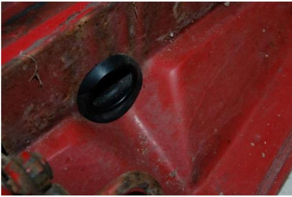
3. If you do not have power windows, remove the plastic plugs in the center of the door and pillar (the holes were already placed there whether you have power windows or not). Repeat the same procedure on the other door.
