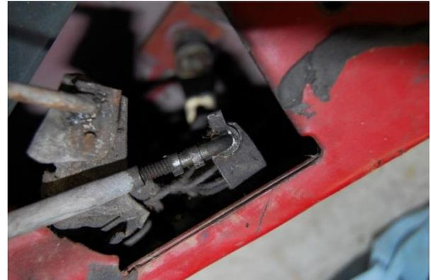
14. If required, lengthen or shorten the O.E. lock linkage horizontal rod at the end link that rotates. In some cases, the O.E. lock linkage vertical rod also requires adjustment to get full travel without bottoming out the door lock actuator rod in the housing.
