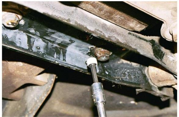
6. Flush the differential with brake cleaner at least twice. Use the brake cleaner to clean the outside of the differential as necessary, then insert the drain plug.
