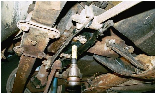
2. A stop is installed on the inside of the 5/8 inch hole saw to prevent drilling into the differential housing. The hole saw is used to cut the strut rod bracket only! Once the hole saw bottoms out against the internal stop, additional pressure may be required to finish cutting the strut rod bracket. Using the 5/8" hole saw, begin to drill into the strut rod bracket. Drill until you have successfully cut the hole in the strut rod bracket and fluid begins to drain from the differential.
