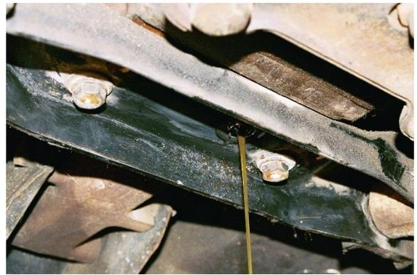
4. Allow the differential to drain.
