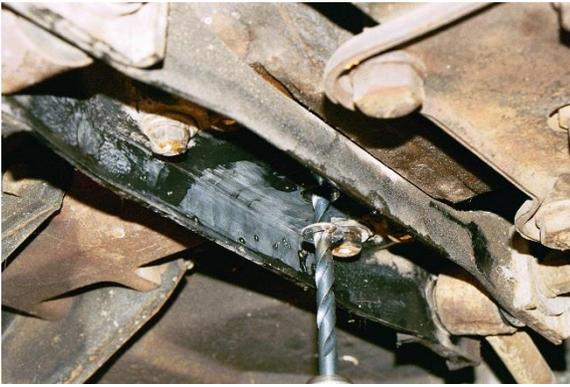
3. Using the 5/16" drill bit with stop, drill into the differential housing until you reach the stop.
