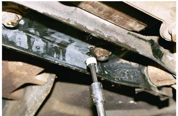
6. Flush the differential with brake cleaner at least twice. Use the brake cleaner to clean the outside of the differential as necessary, then insert the drain plug.
