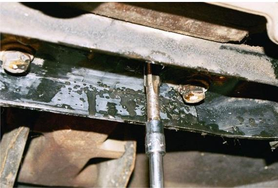
5. Use the 1/8" pipe plug tap to start threading the 5/16inch hole. Try to keep the tap going in straight and back off a quarter turn every two revolutions to clear any chips from the tap- this keeps the threads clean and smooth. The tap should bottom out against the stop.
