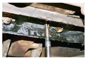
5. Use the 1/8" pipe plug tap to start threading the 5/16inch hole. Try to keep the tap going in straight and back off a quarter turn every two revolutions to clear any chips from the tap- this keeps the threads clean and smooth. The tap should bottom out against the stop.
