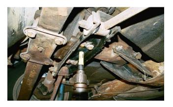
2. A stop is installed on the inside of the 5/8 inch hole saw to prevent drilling into the differential housing. The hole saw is used to cut the strut rod bracket only! Once the hole saw bottoms out against the internal stop, additional pressure may be required to finish cutting the strut rod bracket. Using the 5/8" hole saw, begin to drill into the strut rod bracket. Drill until you have successfully cut the hole in the strut rod bracket and fluid begins to drain from the differential.
