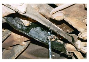
3. Using the 5/16" drill bit with stop, drill into the differential housing until you reach the stop.
