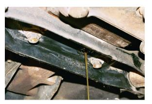
4. Allow the differential to drain.
