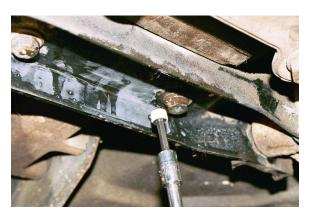
6. Flush the differential with brake cleaner at least twice. Use the brake cleaner to clean the outside of the differential as necessary, then insert the drain plug.
