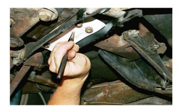
1. Place template on bottom of strut rod bracket around the four bolts. Center punch on the bullseye of the template.
