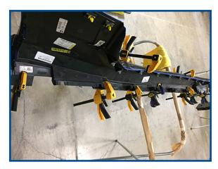
5. Drill your first 1/8" hole through the inside of your OE rocker panel near the end of the Rocker panel closets to the front tire. You should only drill your hole through the OE Rocker panel and inside panel of your Anderson Composites Side Rocker. It is not necessary to drill through the outside (exposed weave); doing so will result in an unsightly exposed hole.
