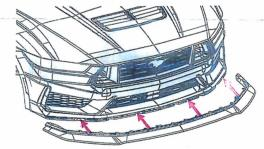
Install supplied (6) screws (W715060-S450B) to attach the splitter to fascia. Tighten screws securely (reference torque 1.7Nm).
