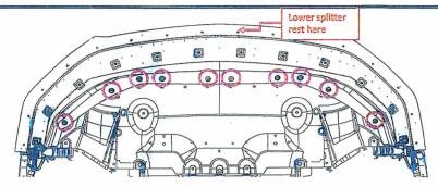
9) Fasten supplied (16) screws (W506843-S450B) between lower splitter and upper splitter. (Reference torque 1.7Nm).
