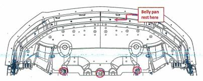
8) Install lower splitter (PR3B-17D997-A-PIA-02) by resting forward edge on upper splitter and installing supplied (10) push pins (W713202-S442).
