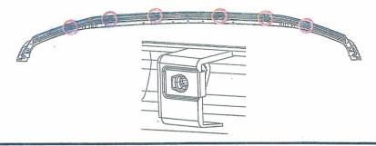
Attach Handling Package Upper Splitter (PR3B-17D997-A-PIA-01) to front fascia by fully engaging (8) snaps.
