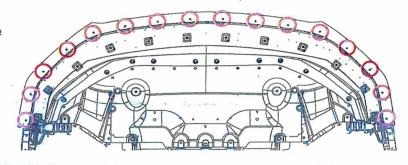
10) Fasten remaining belly pan (22) screws (W715060-S450B). (Reference torque 1.7Nm).
