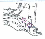
7) Partially re-install belly pan by resting forward edge of belly pan on fascia and installing (3) push pins (W711035-S442) to help hold up belly pan.
