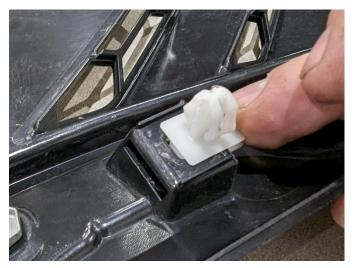
Step 5: Install (4) hood vent T-Studs into the carbon fiber hood vent in the locations noted in Step 3 by clipping them into position.
