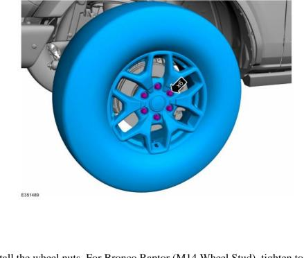
Step 13: Install the wheel nuts. For Bronco Raptor (M14 Wheel Stud), tighten to 200 Nm (147.5 lb-ft).
