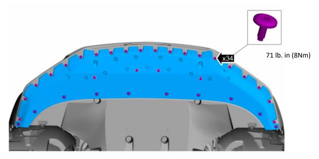
5. Remove the bolts, the screws, push pins, the trim pin and the under engine closeout panel
