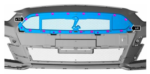
3. If equipped, remove the rivet blinds and the license plate bracket
