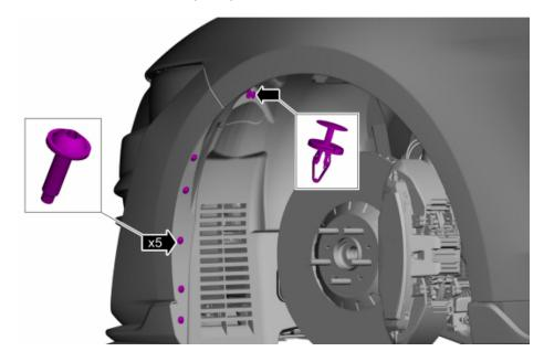
7. On both sides, remove push pins and position the fender liner aside
