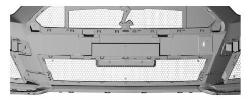
2. Remove the screws, release the tabs and remove the upper radiator grille panel
