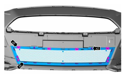
5. Release the tabs and remove the gloss black front bumper insert panel
