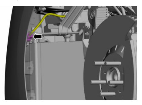
9. On both sides, remove the bolts, trim pin and separate the front bumper cover from the fender bracket
