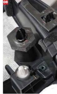
nal door mechanisms is a big job, the mounting of the door to the car could not have been easier. On late-model Mustangs, there is no hinge adjustment possible or required. Two threaded studs exit the door and fit through the
