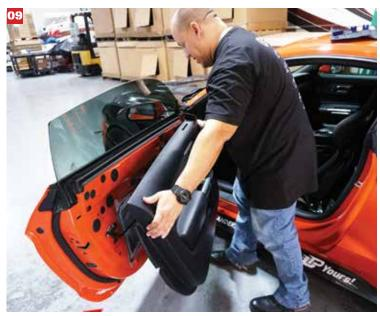
O4 This specialty tool kit from Anderson Composites is designed to work with interior parts that can become scratched or damaged using more standard tools. This tool kit was extremely helpful.
