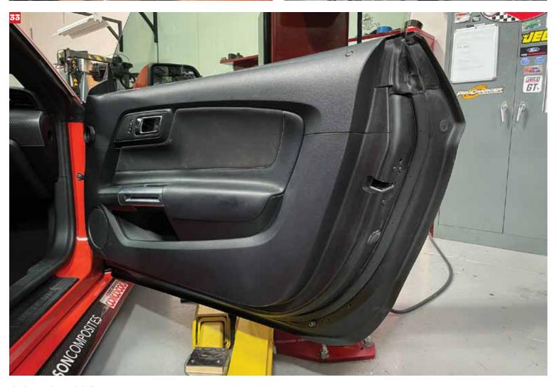
the door can be a real challenge. We removed brackets that connected to the regulator, noting where they fit by photographing the pieces as they come apart. This is one of the more challenging parts of this door swap. The good thing is that the new carbon door is identical to the steel door
