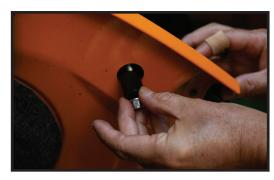
12. Fasten the "dog bone" brackets to each side of trunklid and adjust as needed for best fitment to spoiler.
