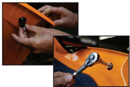
11. Install the "dog bone" brackets using a Torx #30 bit. Do not fully tighten. Repeat for other side.
