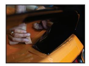
6. Use fishing string to break mounting seal from each side of base. Repeat for other side. Note: String will not pass all way through due to mounting stud.
