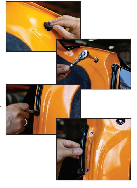
4. Lower the trunklid halfway down and remove the nylock nut with ratchet, the spacer will also fall out through access hole. Repeat on other side.
