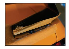
9. Clean dirt off mounting area and remove glue with adhesive removal cup wheel and cordless drill. Vary drill speed and do not over heat the painted surface.
