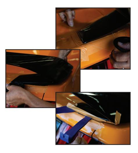
7. Nylon panel removal tools may be used to assist with spoiler removal.
