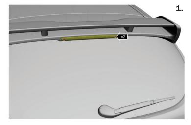
Disconnect electrical harness and rear washer hose from the lens. Remove lens.
