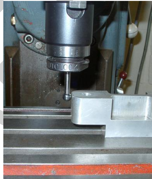
Figure 5-77 - Edge-finder in use on a mill
