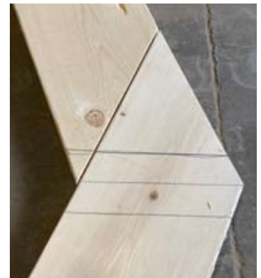
19. Make sure the inside corner is in place and secure with 2 1/2" Zinc screws as shown.
