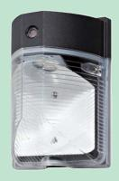
**FEATURES:** Options with and without photocell. Heavy duty die--cast aluminum housing, fully sealed to be dirt and bug proof. High quality shatterproof glass refractor. Internal secondary heat sink to optimize thermal transfer and maximize performance and life of LED. Driver is mounted in direct contact with the casting for a low operating temperature and long life. Easy low cost maintenance and repair. UL, CUL, certified to wet location, DCL Listed.
