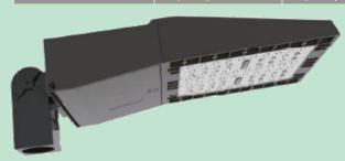
FEATURES: Heavy duty die--cast aluminum housing, fully sealed to be dirt and bug proof. High quality tempered glass optics. Integral secondary heat sink to optimize thermal transfer and maximize performance and life of LED. Driver is mounted in direct contact with the casting for low operating temperature and long life. Polyester powder-coated finish, rust and corrosion proof; stabilized to extreme climate changes without cracking or peeling.
