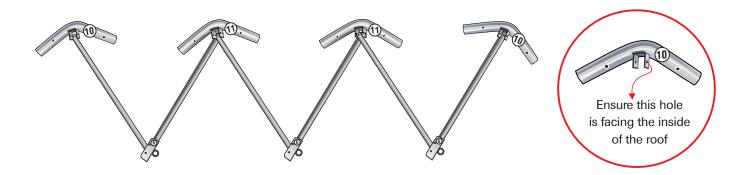
**STEP 4:** Now insert all the poles into the joiners and tighten them with the screws provided. Make sure the concertina grid is on the inside of the roof.
