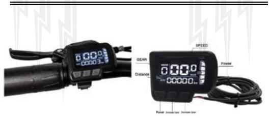
Rotate the throttle to move the bike at the desired speed. It has five different gears. Pushing the +/- buttons the gears change from 1-2-3-4-5. To slow down, push the brake lever and turn the throttle handle anticlockwise. Turn the key to turn off.
