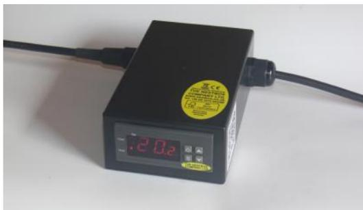
Find a suitable location (such as an accessible shelf), and then connect it to the Bat Box by plugging the connector on the end of the cable coming from the Bat Box into the socket on the side of the Temperature Controller. Lock the connectors together by
