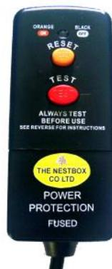
Switch on the system by pressing the reset button.
