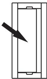
4. Slide the Insert into the box from the bottom. Push it in as far as it will go.
