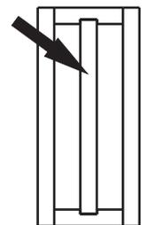
5. Position the Base at the front of the box between the 2 Sides and the Front, leaving a gap at the back for the bats to enter. Nail it in from the 2 Sides.
