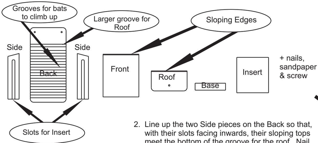
2. Line up the two Side pieces on the Back so that, with their slots facing inwards, their sloping tops meet the bottom of the groove for the roof. Nail from the back into these side pieces.
