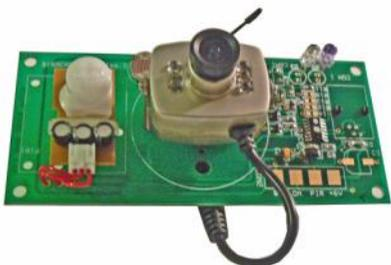
**Circuit Board with Camera**, with cable to connect to Battery Box, and 4 mounting pillars
