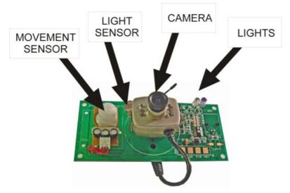
The Circuit Board can be secured in position by making mounting grooves in your box, or using the mounting holes in the 4 corners of the board. These mounting holes are approximately 4mm diameter, and have centres approximately 47mm and 113mm apart (see picture below).
