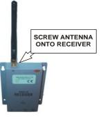
mounted vertically using the screw holes provided, or rested in a horizontal position. Adjust the angle of the Antenna so that it is approximately vertical.
