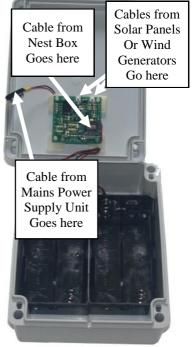
Route all the cables entering the Battery Box through the cable slot in the base of the box. Secure the front of the box using the 4 plastic pegs (which should be inserted fully, and then turned 90° with a screwdriver to lock).
