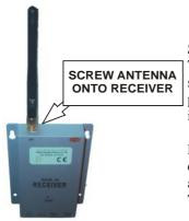
Screw the Antenna onto one end of the Receiver. The receiver can be mounted vertically using the screw holes provided, or rested in a horizontal position. Adjust the angle of the Antenna so that it is approximately vertical.
