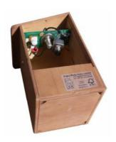
Plug one end of the black cable into the black socket on the circuit board. You may find it helpful to slide the circuit board out slightly to do this.
