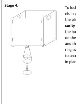
To lock all the panels in place, insert the pin of the **Security Clip** through the hole in the tab on the front panel and then flip the ring over the tab to secure the Clip in place
