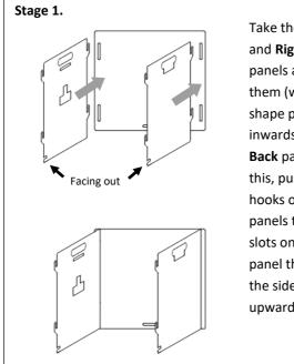
Take the **Left Side** and **Right Side** panels and attach them (with the T shape piece facing inwards) to the **Back** panel. To do this, push the hooks on the side panels through the slots on the back panel then slide the side panels upwards.
