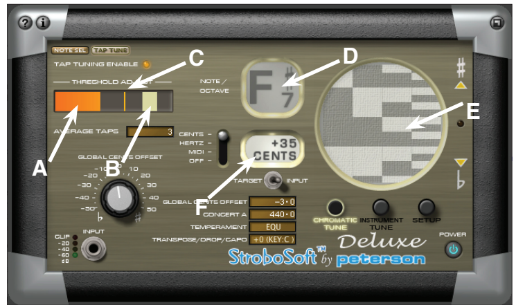
Fig. 3 - StrobeSoft TAP TUNE display screen: A) orange amplitude bar in VU meter; B) white threshold (maximum amplitude) in VU meter [do not exceed]; C) line that indicates the amplitude of the last tap; D) the pitch, sharpness or flatness, and octave of the note; E) the tuning wheel; F) the cents window indicating number of cents sharp or flat of the note.
