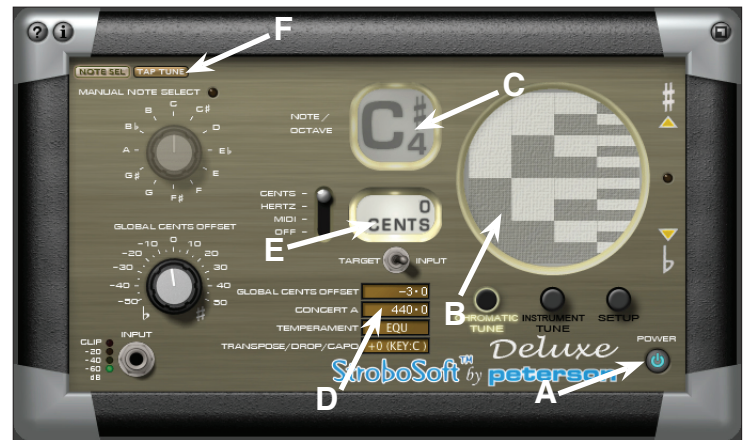
Fig. 1 - StroboSoft default display screen: A ) on-off button; B ) strobe window (when image moves up, the note is sharp; when image moves down, the note is flat); C ) the note window (shows whether natural or sharped note as well as the octave – here showing 4th octave C#; D ) the preset for concert pitch (here showing 440Hz); E ) how many cents sharp or flat the note is; F ) the on-off button to turn on the tap tuning mode.
