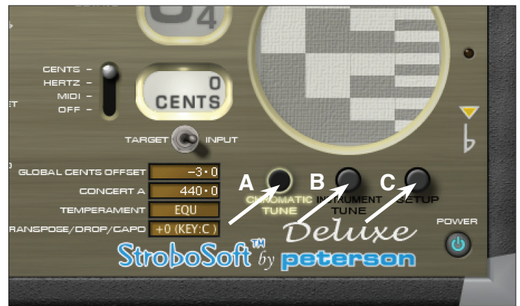
Fig. 4 - Some of StrobeSoft's other functions: A) this button accesses the current default screen; B) this button accesses the screen for several special instrument tunings; C) this button accesses the screen for the oscilloscope, spectrum analyzer, pitch graph, noise filter, and more.
