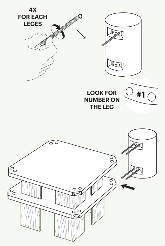
Match up the numbered legs to the numbered sides and slide each leg into place by matching up the dowels and the bolts accordingly.
