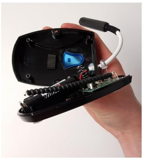
c) Place the base on top of the cover, ensuring the spring fits over the raised pillar on the back of the blue button:
