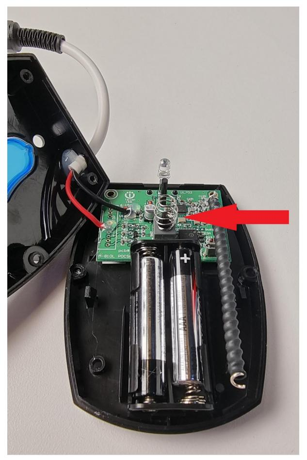
b) Hold the cover with one hand to keep the blue button in place:
