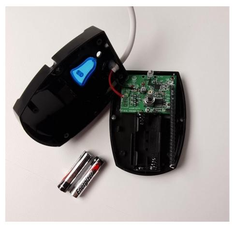
4. Replace the batteries with two new Alkaline AAA batteries.
