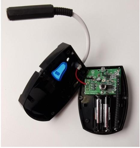
3. Remove the two batteries
