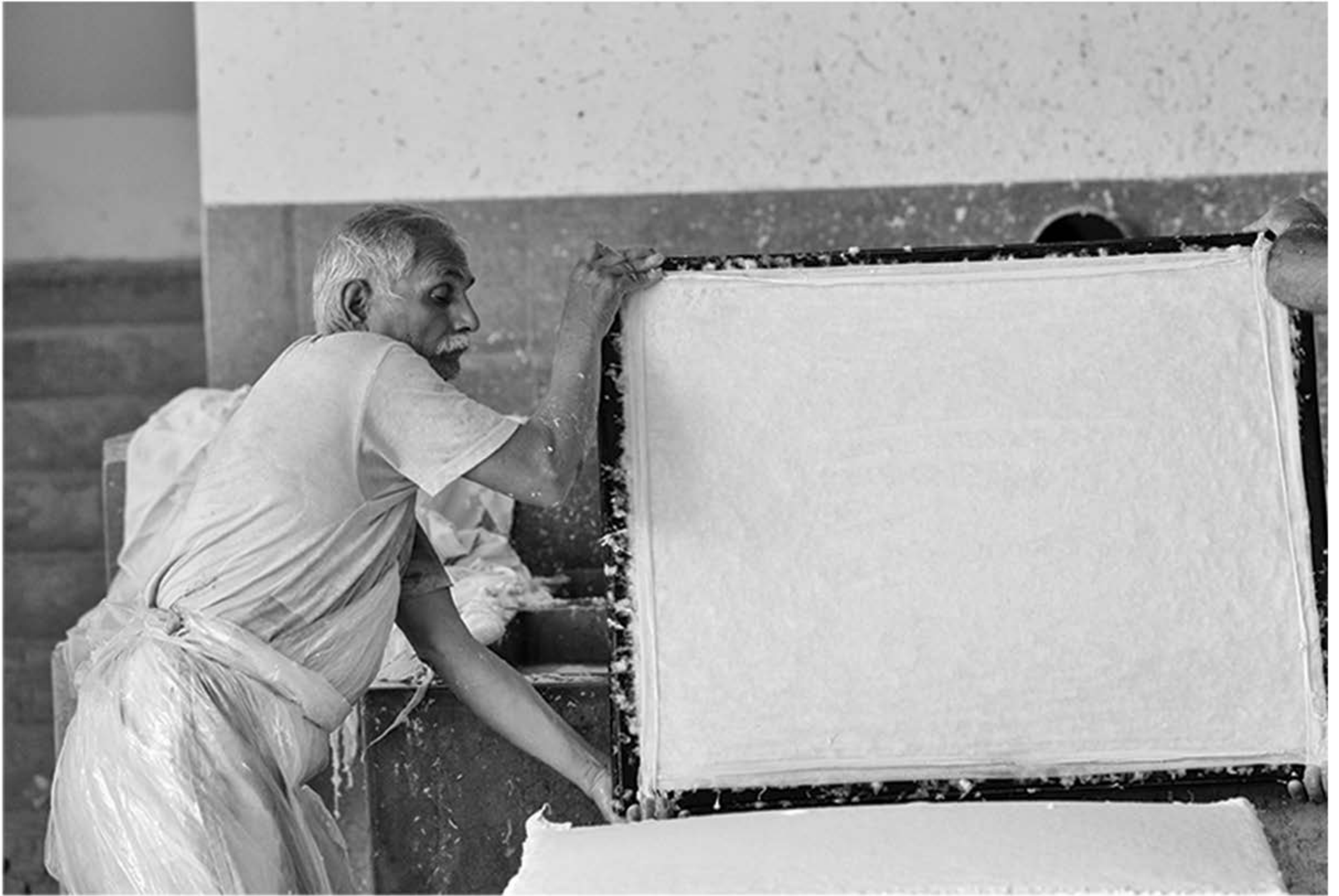
The pulp is drawn into sheets and embedded with seeds.
