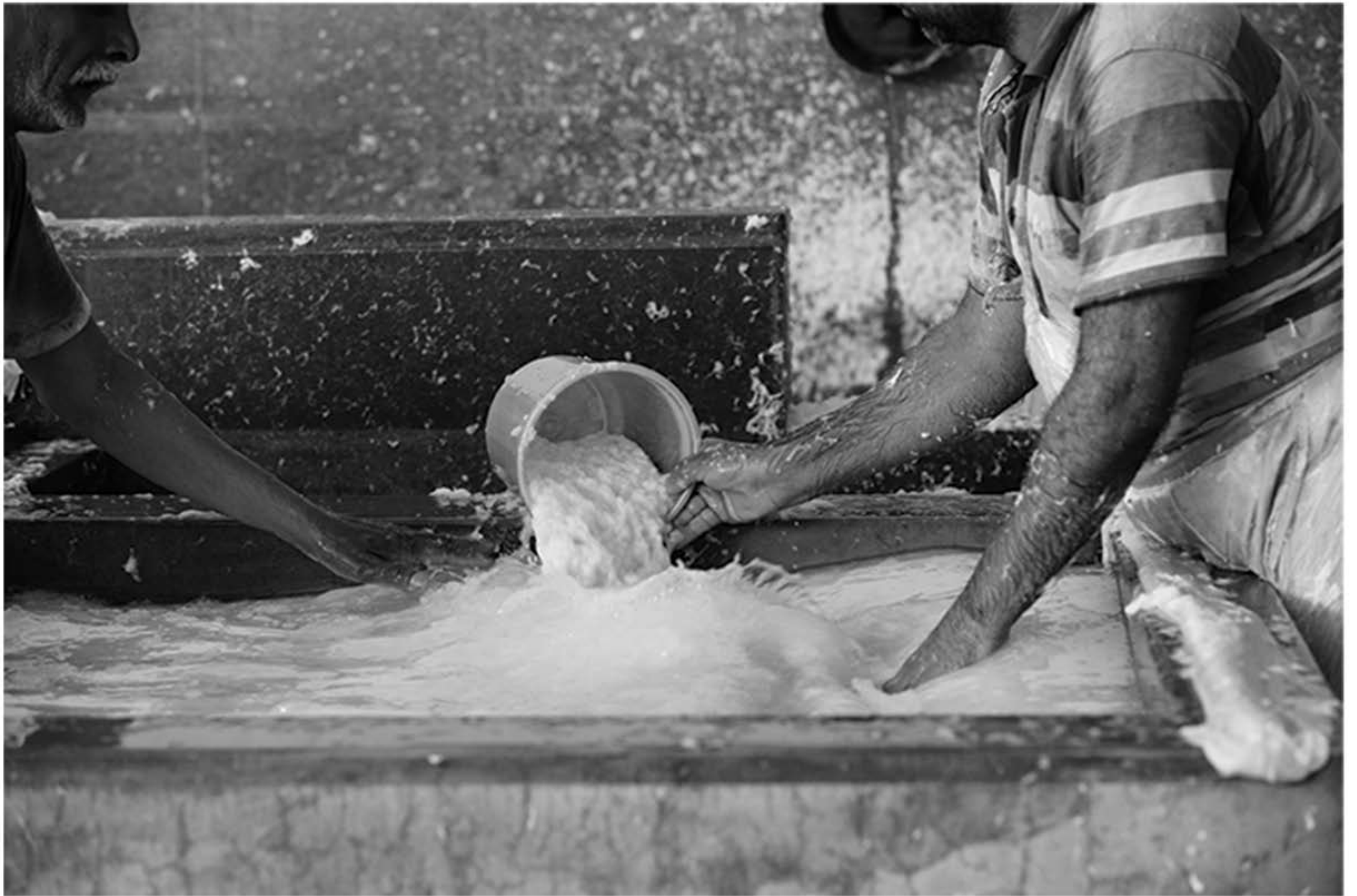
Waste cotton is mixed with water to form a pulp.
