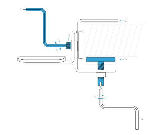
Now place the clamp onto desired surface and use the tool provided A and turn the Locking Bolt D clockwise until tight.
