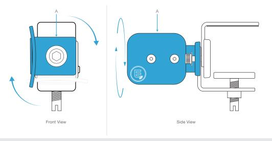
Use the tool provided  $\triangle$  and tighten the Clamp Arms  $\bigcirc$  into position by turning the Central Bolt  $\bigcirc$  clockwise until tight.
