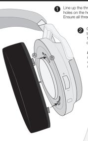
Line up the three clips on the adapter ring A with the three holes on the head unit B, and slot the pad into place. Ensure all three clips are in correctly before continuing.
