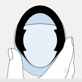
1 Insert earpad mounting ring into inner lip of the earpad
