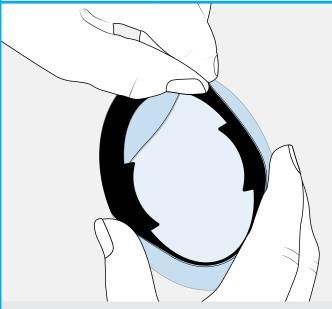
2 Hold the already inserted part in place and further pull the inner lip over the mounting ring
