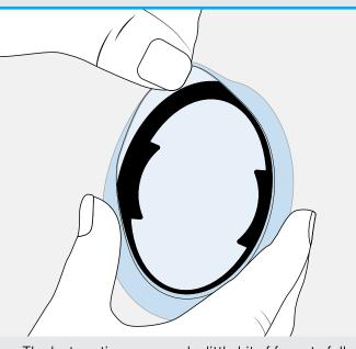
The last section may need a little bit of force to fully insert the mounting ring into the inner lip of the earpad
