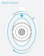
Bring the pad and support ring (A) to the earcup at 90 degrees and twist clockwise until locked in place.
