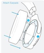
Line up pegs on the pad ring (B) to the holes on the head unit (C), push firmly until flush and pad sits firmly in place.
