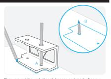
Draw around the rest of each hanger, and mark all screw holes (A). With the sharp pencil poke holes in the paper where you marked the location of the 6 screws (B).
