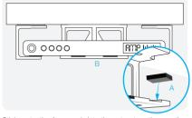
Stick protective foam pads into the cut-out sections on the hanger (A) Stick the third bracket in place to act as a back-stop, and protect your device from sliding too far back (B).
