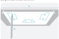
Stick the paper onto the underside of the desk /shelf (A) and use the pencil to mark the locations of the 6 screw holes onto the surface (B).
