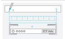
Place the brackets and your device on a flat surface and measure the total width (A). Now mark these measurements on your prepared surface. (B)
