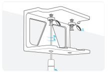
Screw each section into place, make sure to include the decorative screws caps (A). ① For an extra strong fit, use both screws and 3MTM VHBTM tape.
