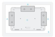
Create a mounting template by arranging the three hanger sections (A) upside down on a large piece of paper (B), along with your chosen device (C).
