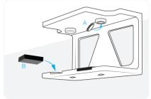
Close the screw caps (A) and stick protective foam pads into the cut-out sections on the hanger (B), hanger is now ready for use.
