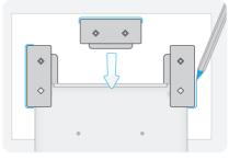
With a pencil draw initial lines around each of the hanger sections, then remove the laptop / device
