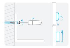
Use a phillips/cross head screwdriver (A) to tighten the screw until you feel resistance, do not over-tighten. If screw caps (B) are provided, attach them now.
