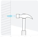
Use a small hammer to gently tap the supplied wall plugs into the hole.
