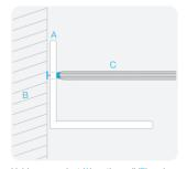
Hold your product (A) on the wall (B) and use a sharp pencil (C) to mark location of the screw holes.
