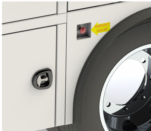
Fig. 4. Street Side Emergency Shut-Off Switch
