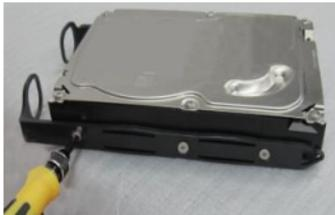
2. Loosen the screws and then open the front panel.
