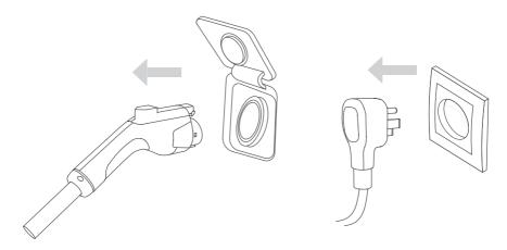
5. Place the dust cover onto the charging connector after use.
