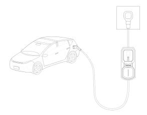
**6.** Remove the charging connector from the vehicle inlet socket when charging is finished, then disconnect the power / charging input plug from the power outlet.
