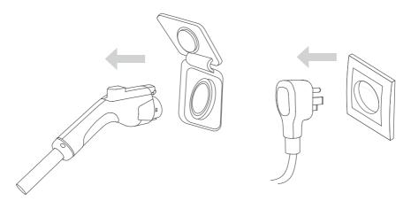
7. Place the dust cover onto the charging connector after use.
