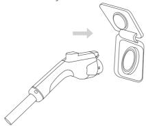
**4.** Remove the charging connector from the vehicle inlet socket when charging is finished, then disconnect the power / charging input plug from the power outlet.
