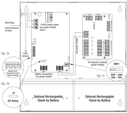
Keep power-limited wiring separate from non power-limited. Use minimum 0.25" spacing.
