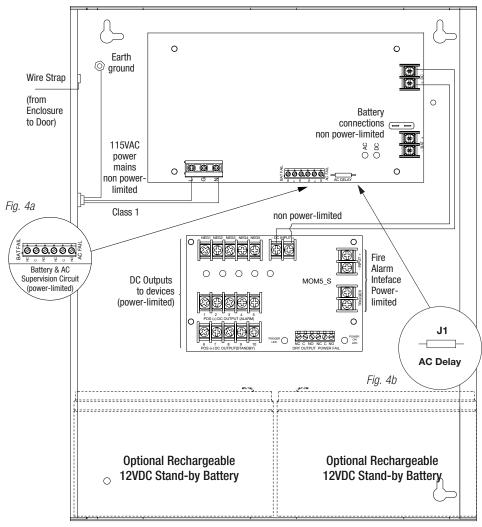
Keep power-limited wiring separate from non power-limited. Use minimum 0.25" spacing.
