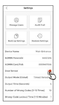
Enable the door sensor\* for a warning when the door is held open longer than the set relock time (see pg. 15) or if the door is forced open. Note that the device cannot distinguish between a door forced open and a door that is held open beyond its relock time.
