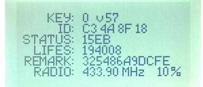
If key data stay empty on LCD it means IR communication doesn't work in this key.
