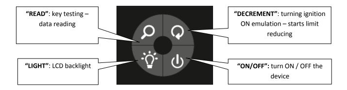
Press "ON/OFF" button to turn ON the device. Insert testing key in to the slot.
