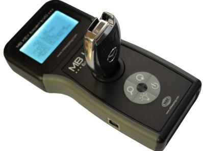
Press "READ" button. Key identification data will be displayed on LCD.
