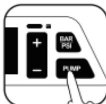
c. BAR、PSI； Short press BAR/PSI button to switch the tire pressure unit
