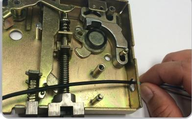
Place REX bracket over **Post** and replace Mounting Tab (B) to secure bracket.
