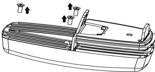
Remove the M4x10 screws with a PH 2 screwdriver, as indicated in the image.
