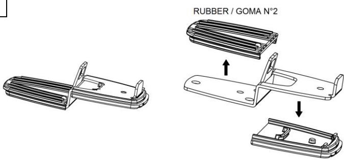
Remove the rubbers N ° 1 and N ° 2 from the Z plate, as indicated in the images.
