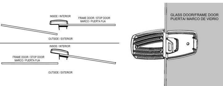
Place the rear part on the frame / stop door or on the swing door according to the opening direction of the door, as shown in the images (the indicated refers in the case that you want to close from the outside, in case of doing it from the inside, the installation direction should be reversed).
