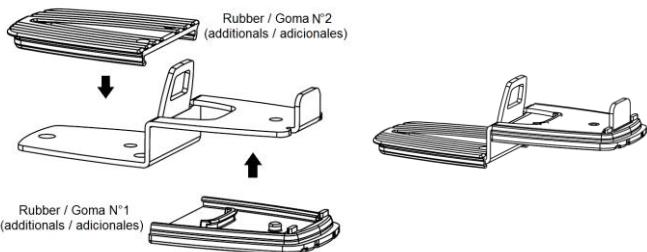
Place the additional rubbers N°1 and N°2 (for use on ½" thickness glass door), as indicated in the images.
