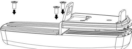
Present the Z sheet with the rubber on the rear part and then fit the M4x10 screws, as indicated in the image.
