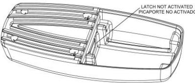
Before installing the front part, check that the latch is not activated, if it is, turn the key and deactivate it. Then place the front part on the back as indicated in the image and turn the key leaving the lock locked.
