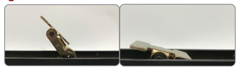
Install the Kit into the back of the Exit Device, ensuring it is laying completely flat and the **Ballscrew Hooks** are in front of the **Device Roll Pin**.
