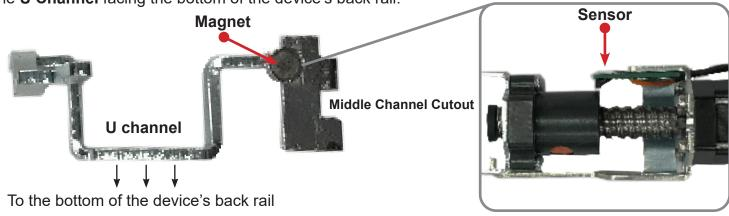
Install the **Magnet Bracket** (50965) at an angle, allowing the **Middle Channel Cutout** to ride on the **Back Rail Extrusion** (See picture 1). Push the **Bracket** down and when seated properly it should be below the **Device's Activating Linkage** (See picture 2).
