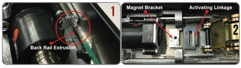
Slide the **Magnet Bracket** (50965) forward and under the **Activating Linkage**. The **Screw Shim** (50990) has **Raised Guides** that must be installed downwards into the **Activating Linkage**.
