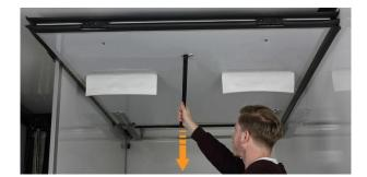
Carefully pull the Cool SmartLift 1D down using the belt.
