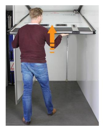
Lift the Cool SmartLift 1D in a horizontal position against the roof.
