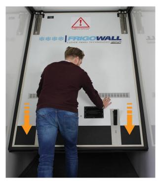
Once the bulkhead is in the desired position, close it downward into the vertical position.
