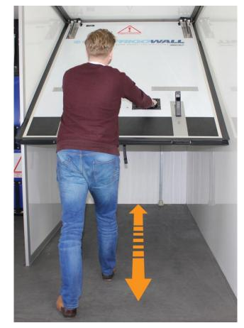
You can now move the Cool SmartLift 1D backwards or forwards into the desired position by simply pushing or pulling whilst it remains at 45 degrees.
