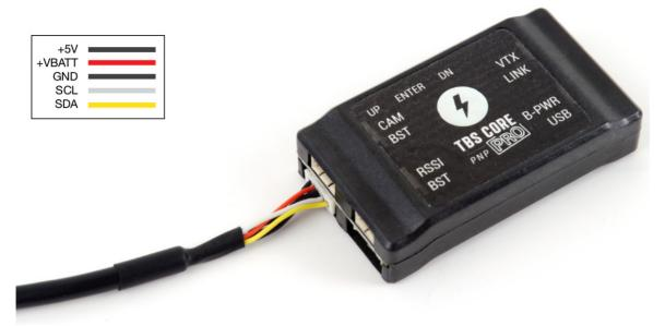
There are two BST ports on the left side of the unit. These can be used to connect a range of compatible modules for the TBS CORE PNP PRO to provide telemetry data. This modular system allows you to custom fit your model depending on your exact needs and weight budget. This is a shared bus, meaning all BST ports use the same physical communication lines. The pin-out is the same for all BST modules.
