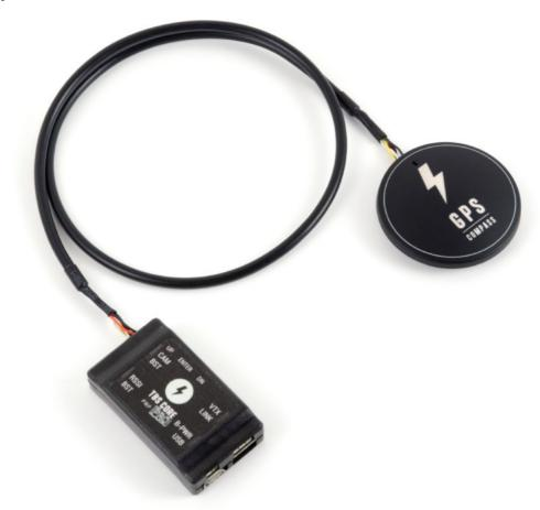
The TBS GPS/COMPASS module (available separately) for the TBS CORE PNP PRO is based on the reliable uBlox GPS sensor and gives you real-time location information in the OSD. It displays an arrow indicating home location (where power was applied), speed (km/h), distance (m) and altitude (m).
