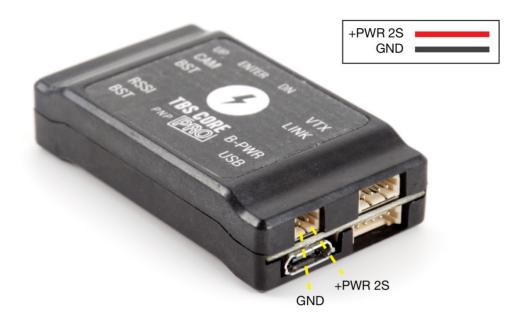
The backup power port is selected when the voltage of the main battery is lower than the backup battery. To add backup power to the system, connect an 2S (7.4V) battery (max. allowed) to the B-PWR port using a 2-pin Molex PicoBlade 1.25 cable (available separately).
