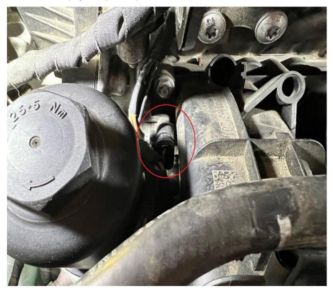
4. Cut the zip tie holding the harness onto the Ecu connector.
