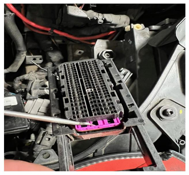
7. Now that the locking tab is out you can locate position 50 (marked white in this image for easier identification) on the connector. This position should be empty. You will need to use a very small pick or paper clip to push the blank out of the connector. Once the blank is out you can install the supplied pin and wire into this position.
