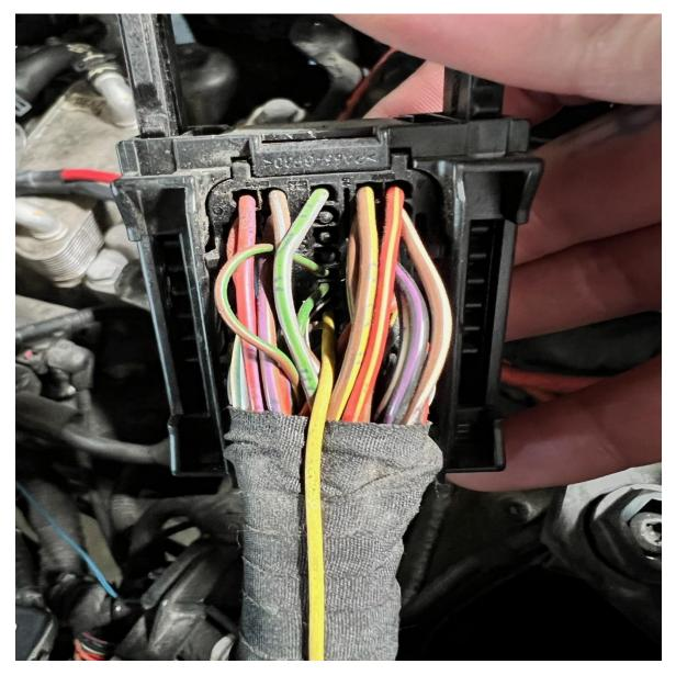
8. Now that your wire is installed you can go in reverse and put your ecu connector back together and plug it back into the ECU.
