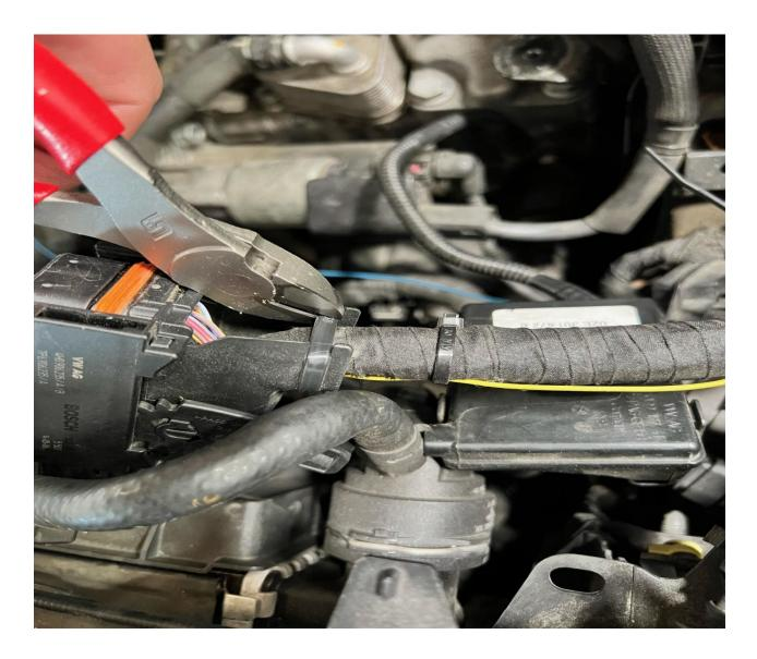
5. Remove the connector cover to reveal the backside of the main body of the connector. This is done easily with a pick tool of your choice.
