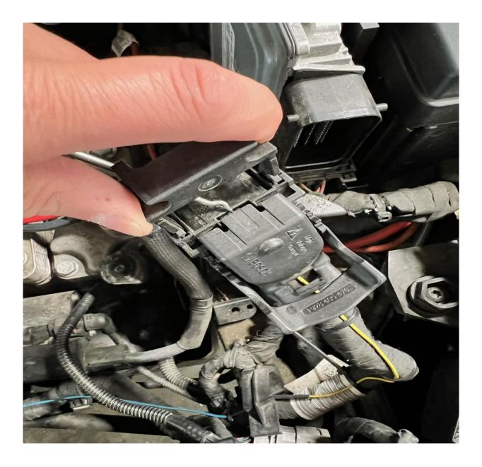
6. Now that your cover is off locate the pink locking tab. You will need to slide this tab out to unlock the pins from the connector. You can use the same pick tool of your choice to do this. It is extremely important that once you slide this locking tab out you do not pull hard on your harness.
