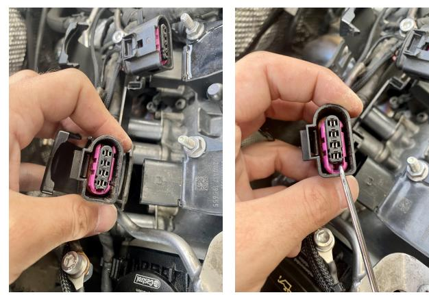
Step 2 - Remove the purple locking tab completely and put it in a safe place that it won't get lost or damaged
