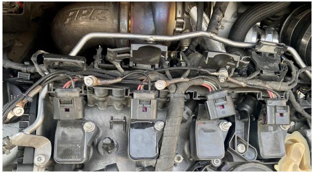
Step 10 - Wire tire any additional or loose cabling together and away from heat then cut off the remaining tails with your cutter tool
