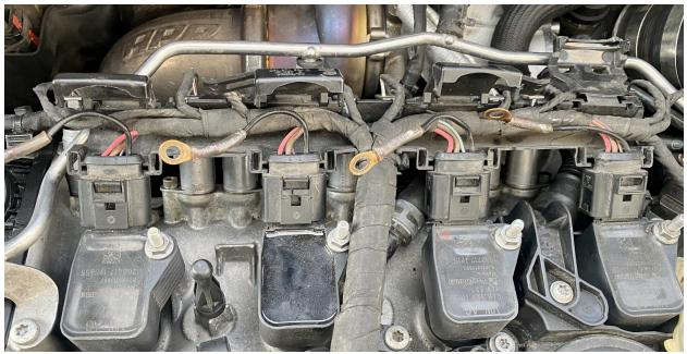
Orient the existing ground wires towards the passenger side of the vehicle as shown above.
