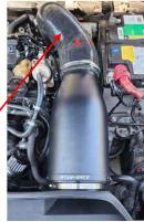
Install turbo inlet pipe with the clamps loosely over the ends of the pipe. Slip turbo end over flange and intake end over AToM Accumulator. Adjust until installation is square and true, then tighten clamps
