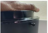
Insert the filter and press down firmly. Use a hand screwdriver to secure the 4x16 screws until they are flush with the case.
