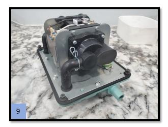
9. Secure new chamber block with old screws and reconnect air tube.
