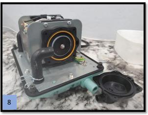
Secure new diaphragm to the magnetic rod with the new nut and washer.
