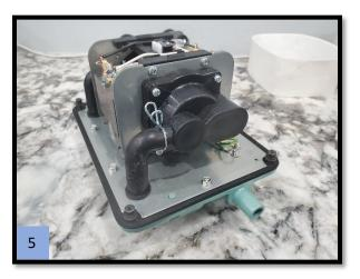
5. Remove the housing and the shroud.
