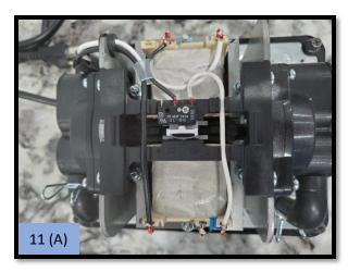
11. (A) If your model has a safety switch, make sure the safety switch is in the run position.
