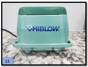
13. Place the housing back on the aerator. The screws holding the housing down should be snug.
