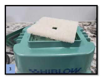
3. Replace the old air filter with the new air filter.
