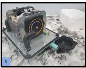
6. Remove the four screws securing the chamber block. Then save the screws for later. Disconnect the air tube.
